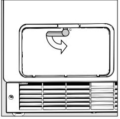
■ Turn the cover lock downwards to the vertical position.
